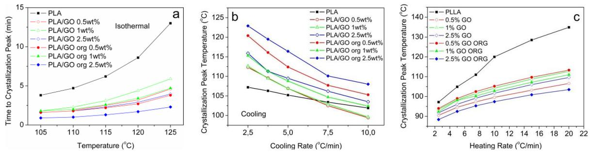
**Figure 3.** (a) Time to peak vs temperature for isothermal crystallization of PLLA and the nanocomposites. (b)  $T_c$  vs cooling rate for crystallization from the melt. (c) Cold crystallization peak temperature of amorphous nanocomposites as a function of heating rate.
