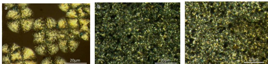
**Figure 5.** Spherulitic morphology of (a) neat PLLA during isothermal crystallization at 120°C, (b) PLLA/GO 0.5wt% at 125°C and (c) PLLA/org-GO 0.5wt% at 125°C
