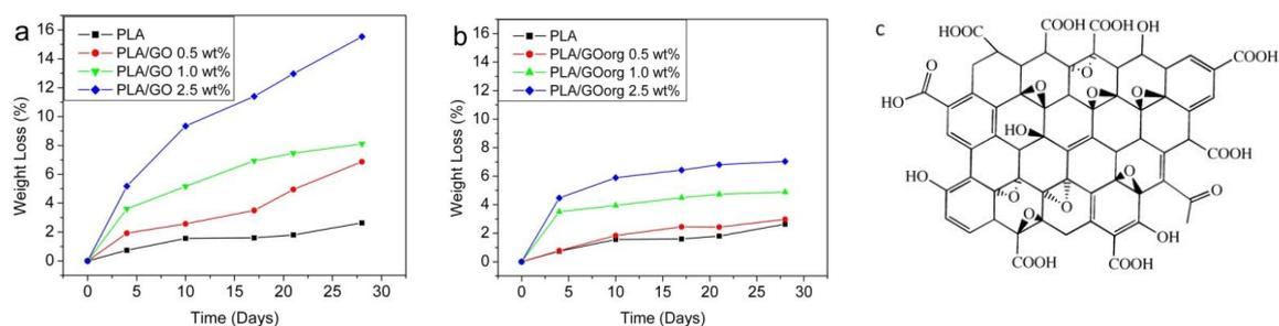
Figure 7. (a) Weight loss vs time of enzymatic hydrolysis for PLLA/GO and (b) for PLLA/org-GO nanocomposites. (c) Chemical structure of Graphene Oxide.
