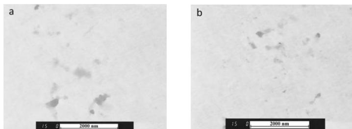
**Figure 1.** (a) TEM photo for PLA/GO 2.5wt% and (b) TEM photo for PLA/org-GO 2.5 wt% nanocomposites
