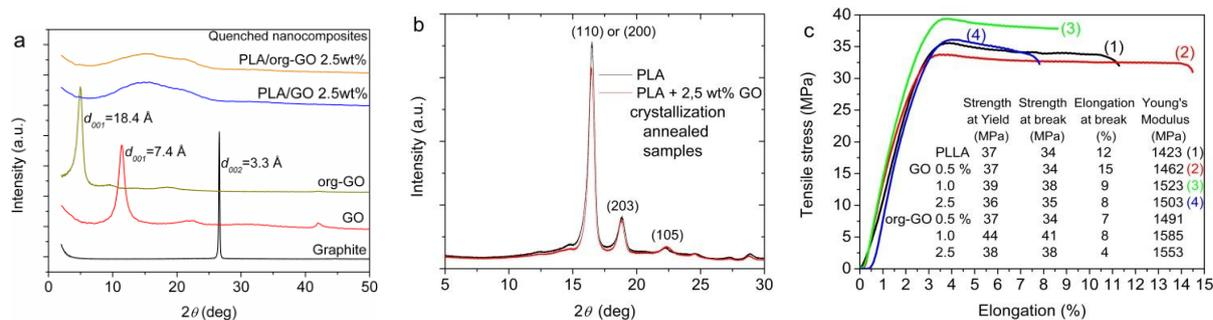
**Figure 2.** (a) WAXD patterns of graphite, GO, org-GO and quenched nanocomposites with 2.5 wt% GO or org-GO. (b) WAXD patterns of PLLA and PLLA/GO 2.5wt% after crystallization annealing. (c) Stress-strain curves for PLLA and PLLA/GO nanocomposites. Tensile properties are listed in the table in the inset.
