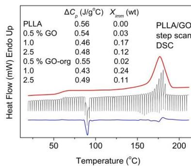
**Figure 4.** Step Scan DSC traces for the quenched PLLA/GO 2.5wt% nanocomposite.  $\Delta C_p$  and  $X_{imm}$  values for PLLA, PLLA/GO and PLLA/org-GO nanocomposites are listed in the table in the inset.
